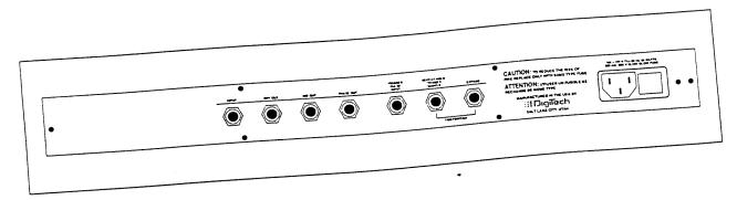
BYPASS For use with a momentary to ground footswitch. Toggles the signal bypass on and off.
