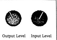
For example, if the INPUT LEVEL is set to the right of center (1 o'clock), set the OUTPUT LEVEL an equal amount to the left of center (11 o'clock).
